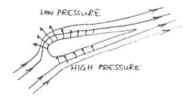
The aerofoil shape of the canopy, based on the wing of an aeroplane, is designed to have minimal resistance with maximum lift capabilities (Diagram). Gliders, having no engine, rely on gravity and a downward tilted wing to provide forward movement. The canopy of the paraglider, when inflated by the air flowing into the open leading edge cells, produces an aerofoil.
